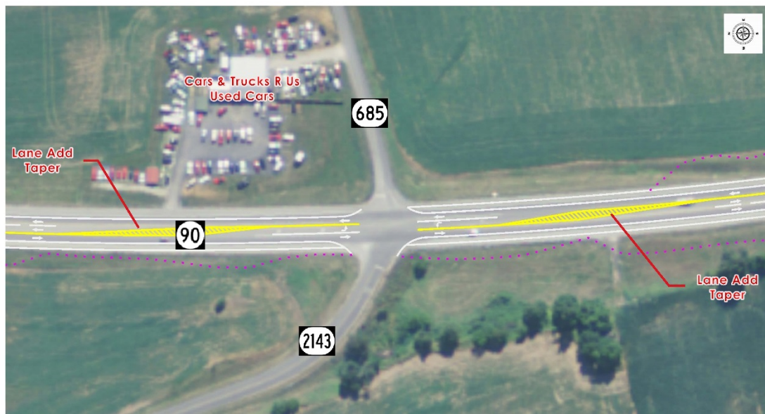
Figure ES-3: Left Turn Lanes on 2+1 Roadways (KY 90 intersection at KY 685)
