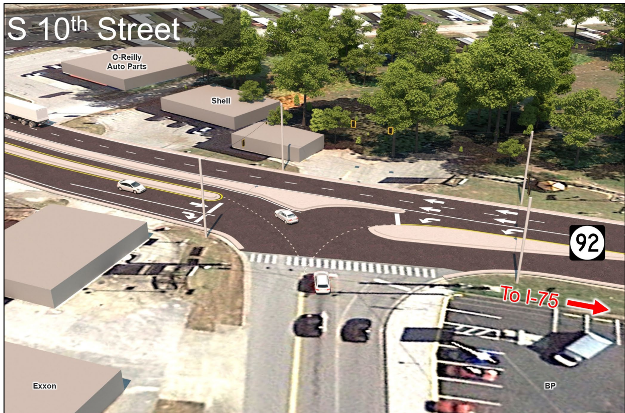
Figure 25: Green T Concept at KY 92 / S. 10th Street Intersection (Looking South)
