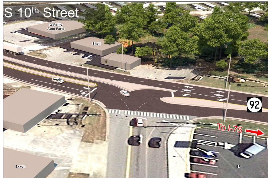
Figure ES-3: KY 92 Concept 2 – Green T Intersection at S 10 th Street (Looking South)
