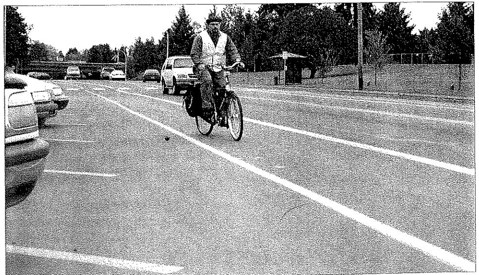
Back-in angle parking with a bicycle lane as a buffer in Vancouver, WA. (Photo: Courtesy Todd Boulanger 2004)
