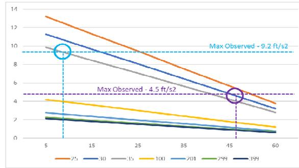
Based on the graph it seems that the MPR-35 class more closely aligns with the observed values - so as most passenger cars will be in the 25/30 categories it might be best to apply a Beta factor to recreate that type of behavior in the 25/30 classes.
