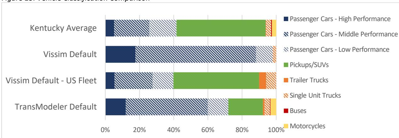
The KY VIN data analysis resulted in a base vehicle distribution that is representative of typical conditions throughout the state. From this distribution, a recommended vehicle composition and a range (providing variance in each direction) were developed. In microsimulation, vehicle composition is often categorized by
