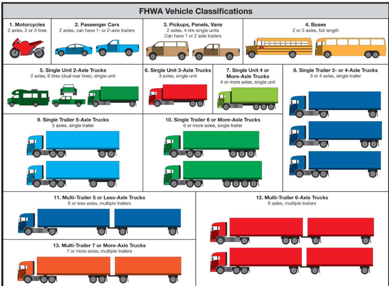
Within microsimulation modeling, the vehicle classification is typically divided by vehicle type and performance and is not directly correlated with the FHWA classification count breakdown; however, the 13-class breakdown can be informative to differentiate or validate the available vehicle deviations within the software. **Table 6** shows the breakdown of vehicle classifications within a typical microsimulation and how that relates to the
