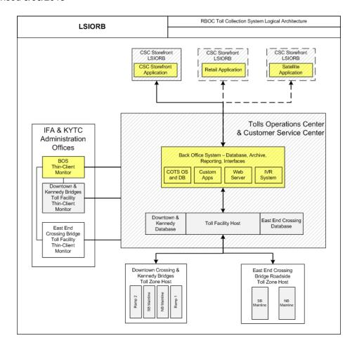
Figure B.2 - RBOC Logical Architecture
