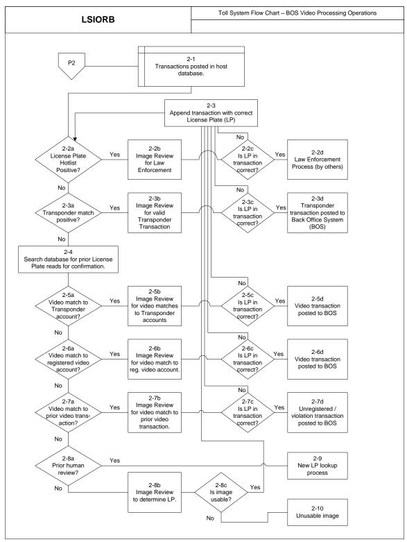
Figure B.4 - Video Transaction Processing
