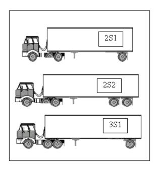
(LSIORB Class – Large Truck) FHWA Class 8 — 3 to 4 Axles, Single Trailer
