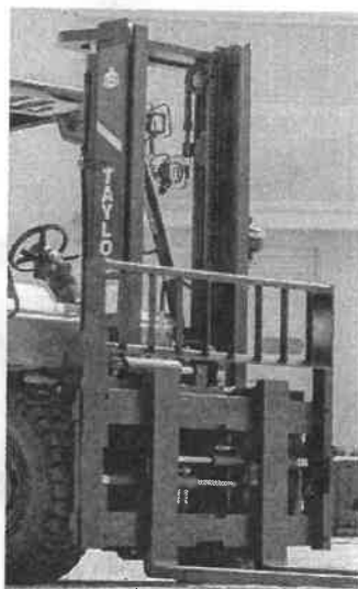
Durable Nested I-beam Design Yields Optimal Visibility
