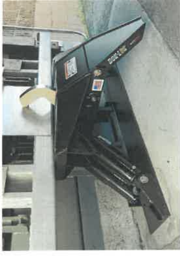
Hook secures intermodal container chassis and Rear Impact Guards (RIGs) with obstructions
