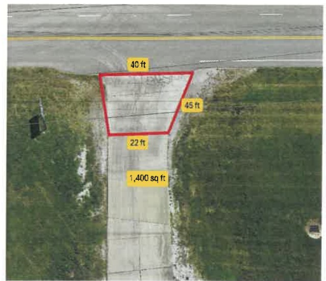
Concrete replacement area
