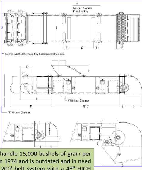
The current conveyor configuration is set up to handle 15,000 bushels of grain per hour on a 30" belt. The conveyor was installed in 1974 and is outdated and in need of replacement. This project will replace the 1200' belt system with a 48" HIGH ROLLER enclosed system. All conveyor legs will be replaced along with the grain cell containing the load out spout. Grain loading on barges will increase by 150%.
