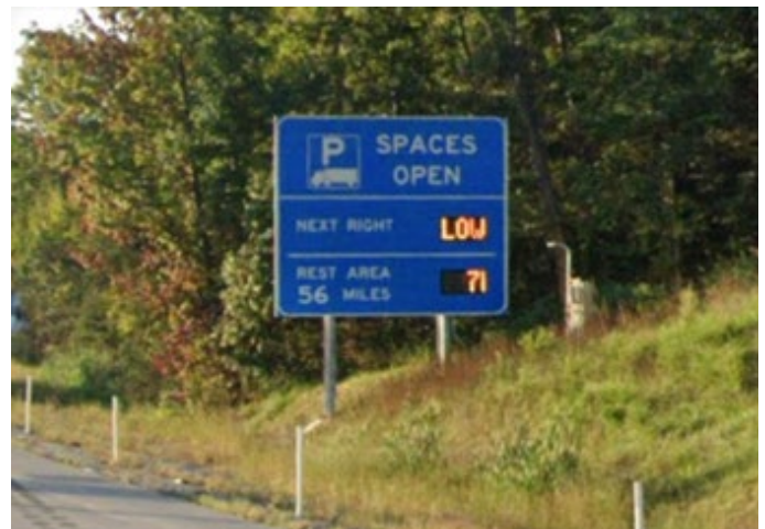
Figure 9-1. TPIMS Sign on I-65 (Bullitt Co.)
