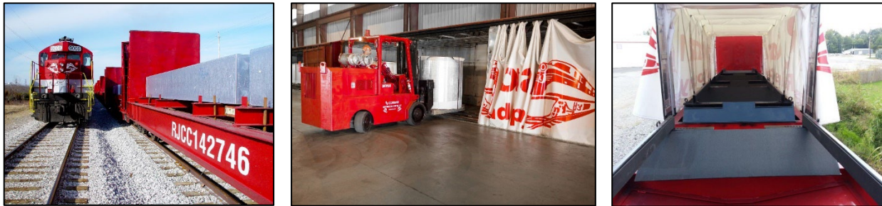
Figure 7: Inbound aluminum ingots and outbound coils at SUDC on specialty cars
