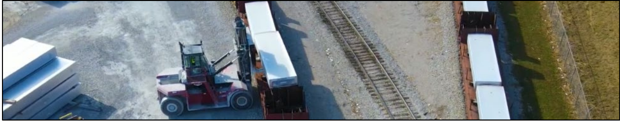
Figure 8: Unloading of aluminum ingots from railcars at the aluminum facility
