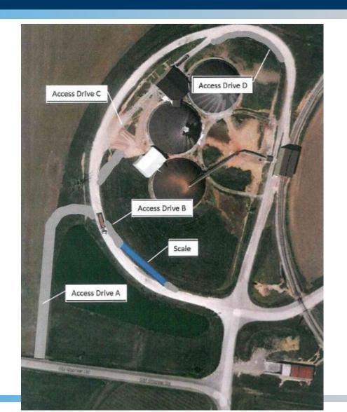
Proposed project would install new automatic scale at a new location that will provide more efficient movement of trucks. Project will also include adding an access drive to divert traffic from busy intersection and sections of current access drives widened to allow two lanes of traffic, increasing efficiency of the operation and reduced idle times.
