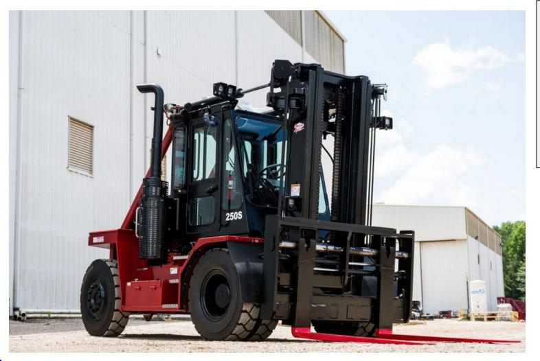
Proposed project would purchase new 25,000 lb. forklift to handle metals (aluminum and steel) for both placing in storage and loading for outbound. New forklift would improve fuel consumption, improve safety and standards, savings on New forklift maintenance. would replace 2014 model with limited availability of replacement parts.
