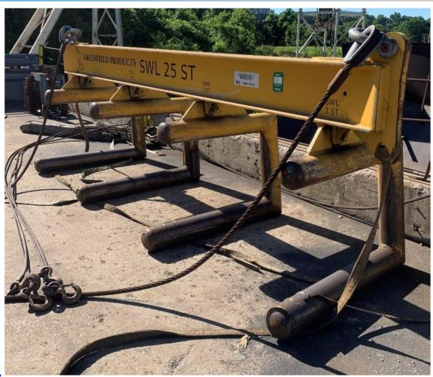
Project will design and construct new spreader bar and coil hooks for unloading different size wire coils from barges. Current equipment is wearing out and is not compatible with the different sizes of wire coils handled by the riverport.
