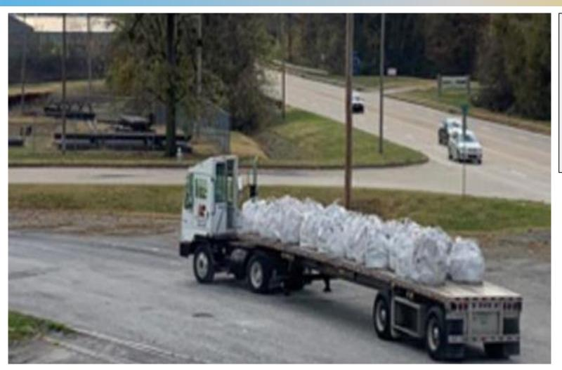
Project would purchase a 48-foot, spring slider, steel chassis flatbed trailer to replace rented trailer. Trailer is used to distribute supersacks arriving by barge into multiple port owned warehouses before distribution to the region. Purchase of trailer would create redundancy by avoiding days when a flatbed trailer is not available to rent.
