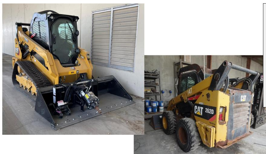
Project replaced existing 2014 model used in daily operations with a new compact track loader. Old track loader has 11,000 hours and due to highly corrosive commodities moved and harsh operating environment, equipment suffered premature failures and limited life span. New compact track loader provides emissions improved standards, improved fuel consumption, improved safety standards and savings on maintenance.
