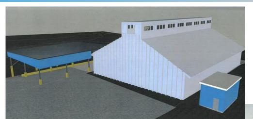
ORA recently purchased the disused property and rehabilitated existing structures. This project would be 2<sup>nd</sup> phase to install new electric and build an overhang dock area for loading out during all conditions prior to being able to lease out facility for bulk storage.
