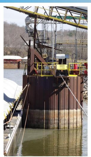
Project installed barge positioning winch system that through a remote control will shift a barge when loading/unloading more efficiently and safer than the current tug winch system.
