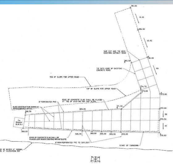
Project would stabilize and concrete the bulk loadout dock. Area is subject to soft soils and saturated ground. When loading materials, trucks dumping in this area are getting stuck and contaminating material being staged. Project would allow for sufficient drainage and provide concrete stabilization for operations.
