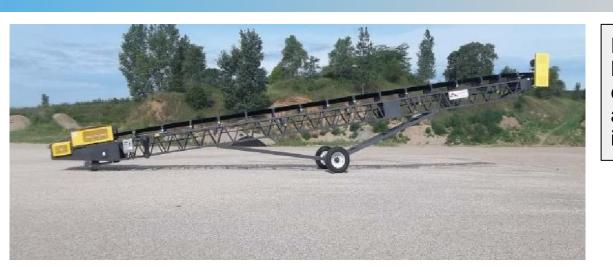
Project would purchase Triple Stack Portable Transfer Conveyor, Large Wheel Loader, and Radial Stacker to allow Riverport to continue current operations consisting of loading coal ash from the adjacent rail line facility. Also allow expansion of operations to include agricultural transport.
