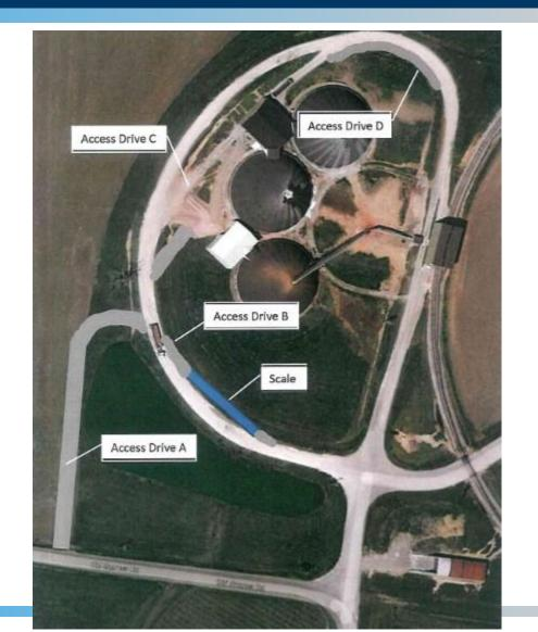
Project installed new automatic scale at a new location that provides more efficient movement of trucks. Project also includes adding an access drive to divert traffic from busy intersection and sections of current access drives widened to allow two lanes of traffic, increasing efficiency of the operation and reduced idle times.
