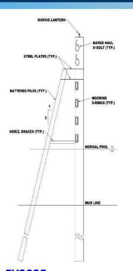
Project would install three mooring dolphins to facilitate the staging of additional barges. The mooring dolphins will provide efficient access for the movement of barge traffic without delaying current operations at the port.
