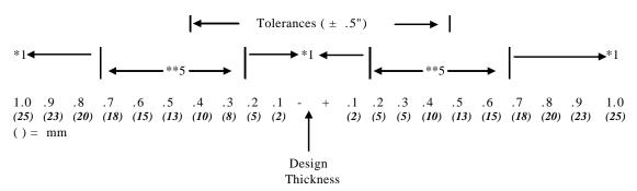
THIS GRAPH SHOWS TOTAL NUMBER OF THICKNESS MASUREMENTS REQUIRED FOR BITUMINOUS PAVEMENT CORES. REFER TO SECTION 4.1
