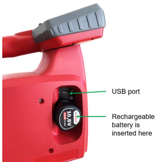
Insert the rechargeable battery on the side of the LTL3000/LTL3500.
