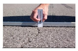
(p2) Rutting – Outside wheel path at 0 feet (p3) Rutting – Outside wheel path at 100 feet
