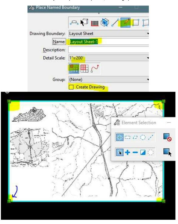
**Step 3:** Create the drawing. This menu, seen below to do so, is found by clicking on the arrow underneath the "Named Boundaries" button. Navigate to the boundary just placed, right-click on it, and select "Create Drawing". A dialogue box appears. First, change the name of the sheet as needed. Review all other properties. Lastly, click "OK" and the Layout Sheet will be created, with the layout map.
