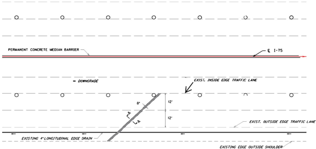
**PERMEABLE PAVEMENT DRAIN DETAIL**
