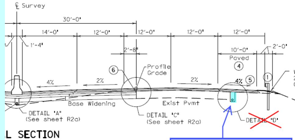
Use existing edge drain--do not remove & replace
