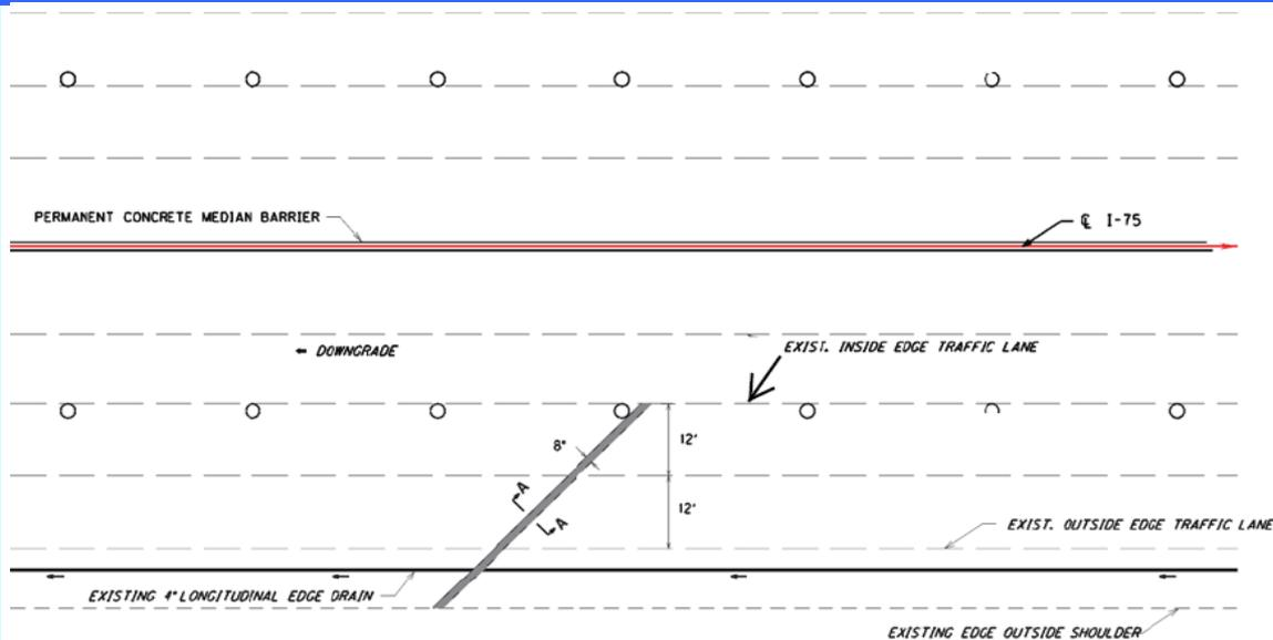
PERMEABLE PAVEMENT DRAIN DETAIL
