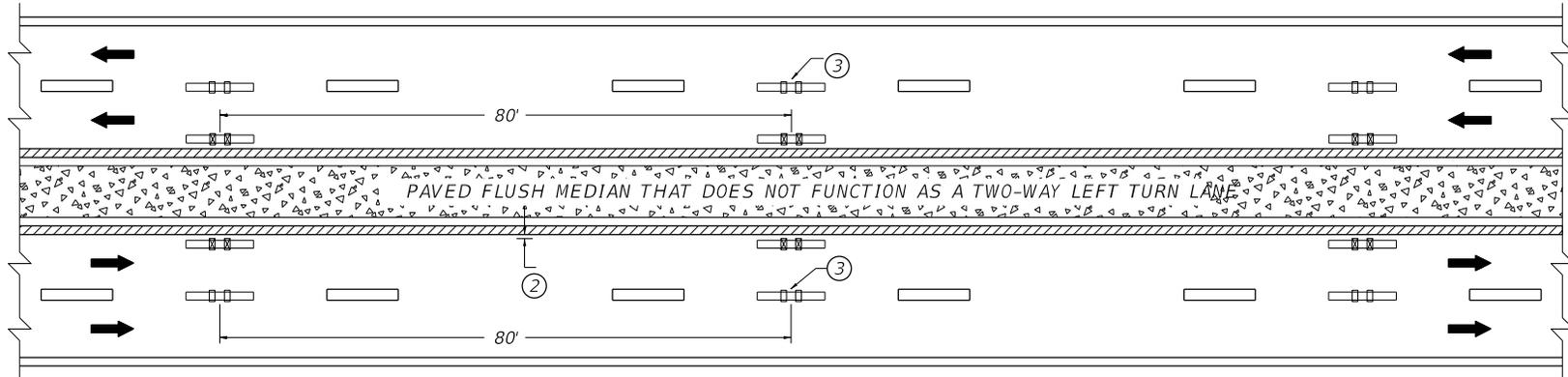
ARRANGEMENT "D" (DIVIDED HIGHWAY WITH PAVED FLUSH MEDIAN THAT DOES NOT FUNCTION AS A TWO-WAY LEFT TURN LANE)
