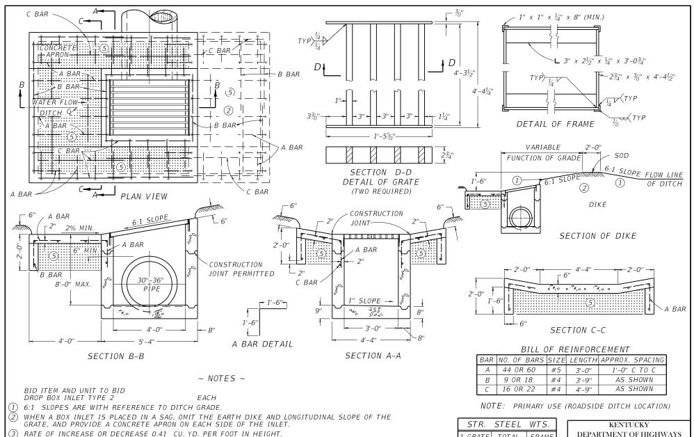
DEDUCT APPROX. 0.2 CU. YD. OF CONCRETE FOR A 30" PIPE AND 0.3 CU. YD. OF CONCRETE FOR A 36" PIPE. COMPACT THIS VOLUME WITH D.G.A. BASE OR GRAVEL BASE AND INCLUDE IN THE UNIT PRICE OF THE BOX.
