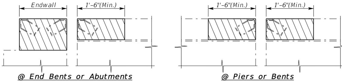
Note: Remove X-Hatched Areas of Concrete & Expansion Device.
