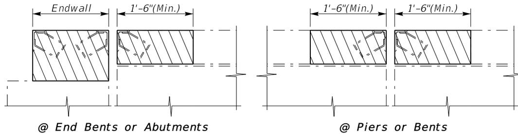
Note: Remove X-Hatched Areas of Concrete & Expansion Device.
