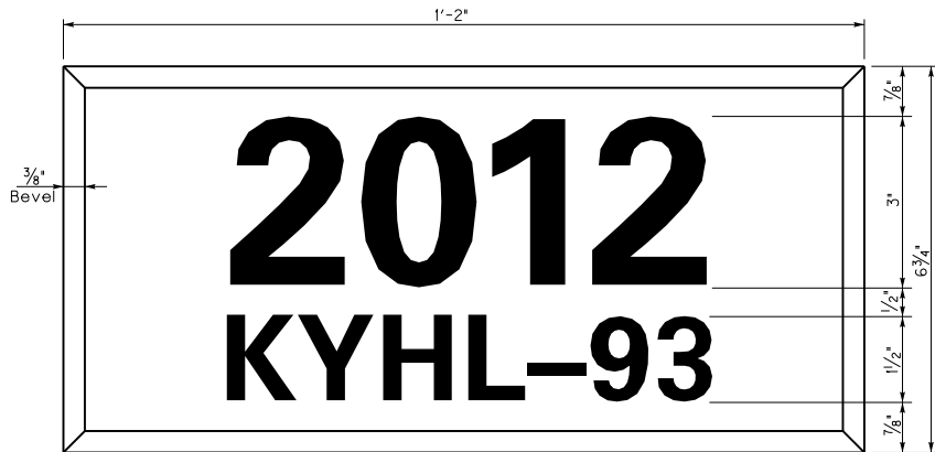
STENCIL FOR YEAR AND DESIGN LOADING When year only is used place year in center of plate
