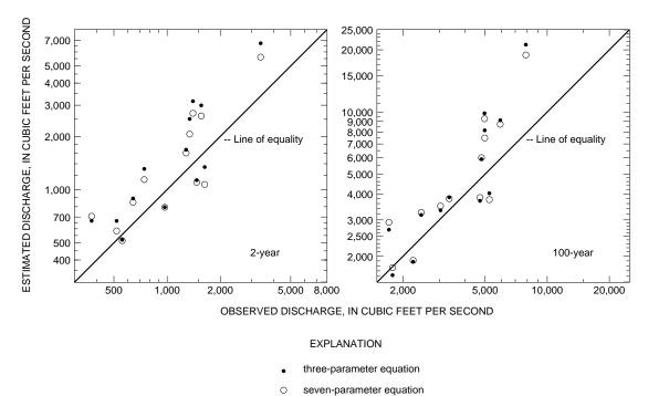
Figure 6. Comparison of 2- and 100-year observed peak discharge to peak discharges estimated using the three- and seven-parameter nationwide regression equations for urban basins in Jefferson County,
