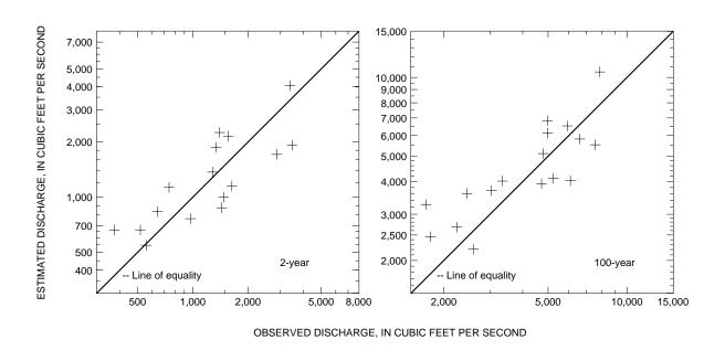
**Figure 7.** Comparison of 2- and 100-year observed peak discharge to peak discharges estimated using the regression equations for Jefferson County, Kentucky.
