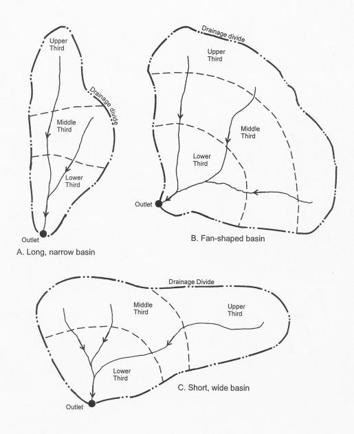
Figure 8. Schematic of typical drainage basin shapes and subdivision into thirds (from Sauer and others, 1983).
