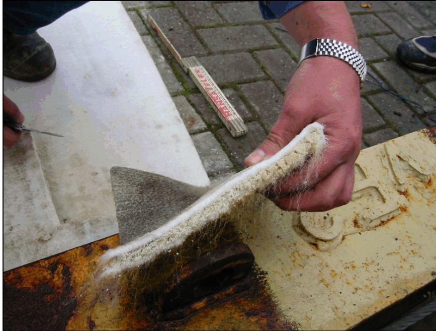
Figure 11.17. Close-up photo of SandMat™ geocomposite blanket.
