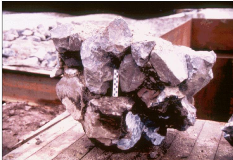
Figure 12.19. Conglomerate produced by spot grouting.
