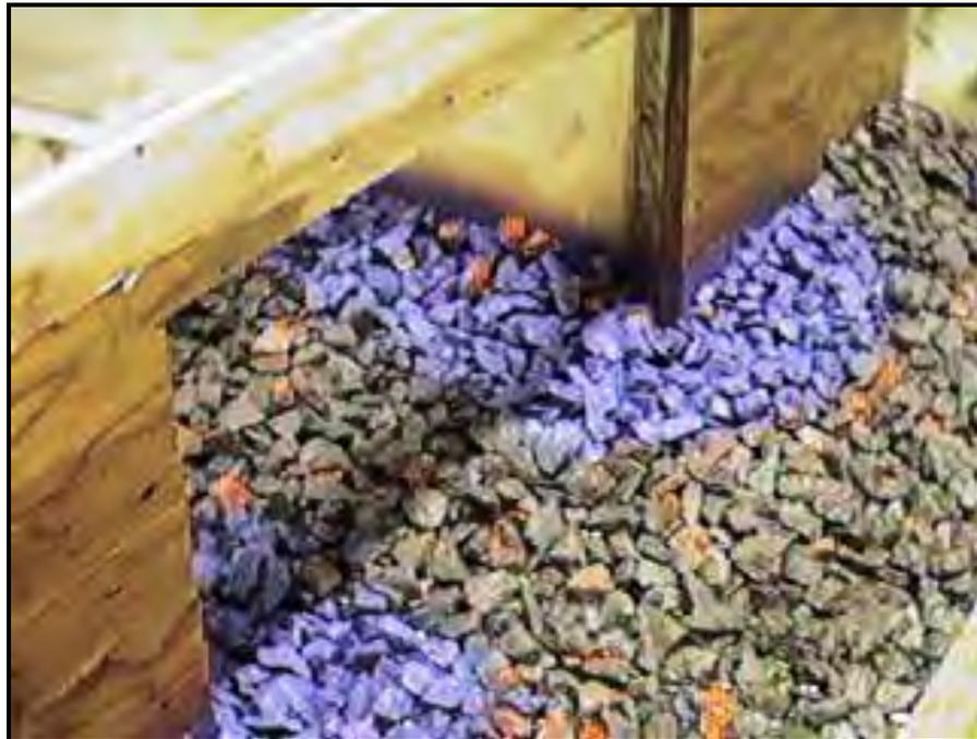
Figure 18.6. Riprap scour protection with a rectangular model (Kerenyi et al. 2003).
