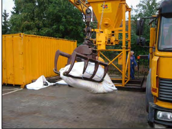
Figure 11.20. Handling a one-tonne sand-filled geotextile container.
