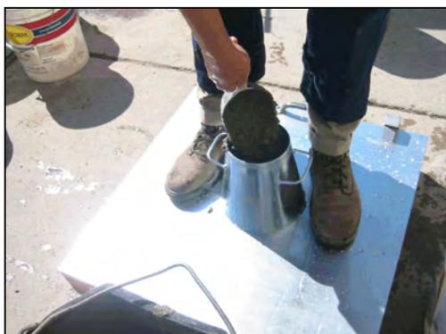
a. Slump cone and test table
