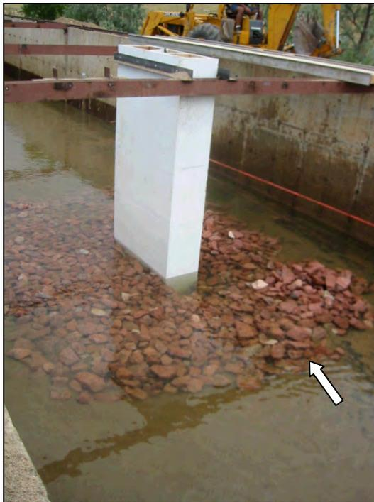
Figure 11.14. Riprap armor over geotextile containers.
