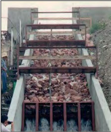
Figure 5.3. Test set up for 1994,  $d_{50} = 1.27$  ft (386 mm).
