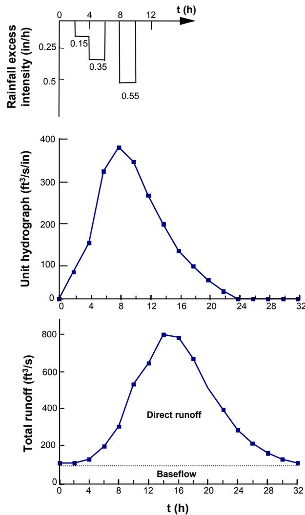
Figure 6.18(CU). Example of hydrograph synthesis
