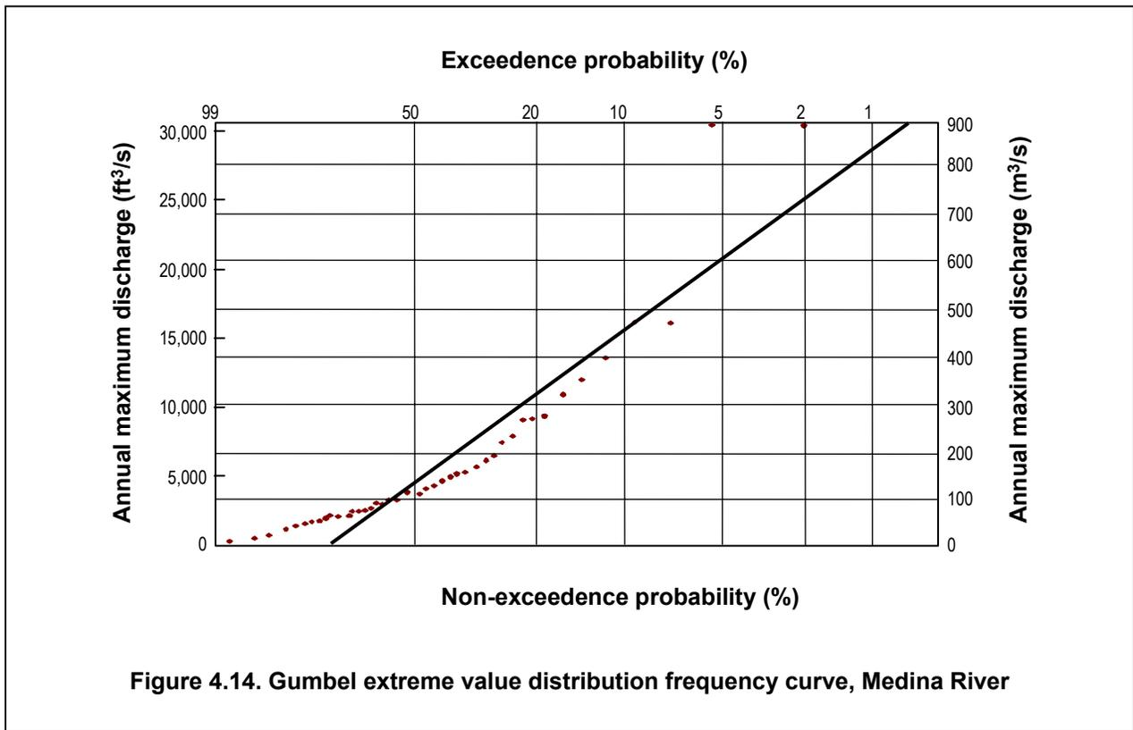
Figure 4.14. Gumbel extreme value distribution frequency curve, Medina River
