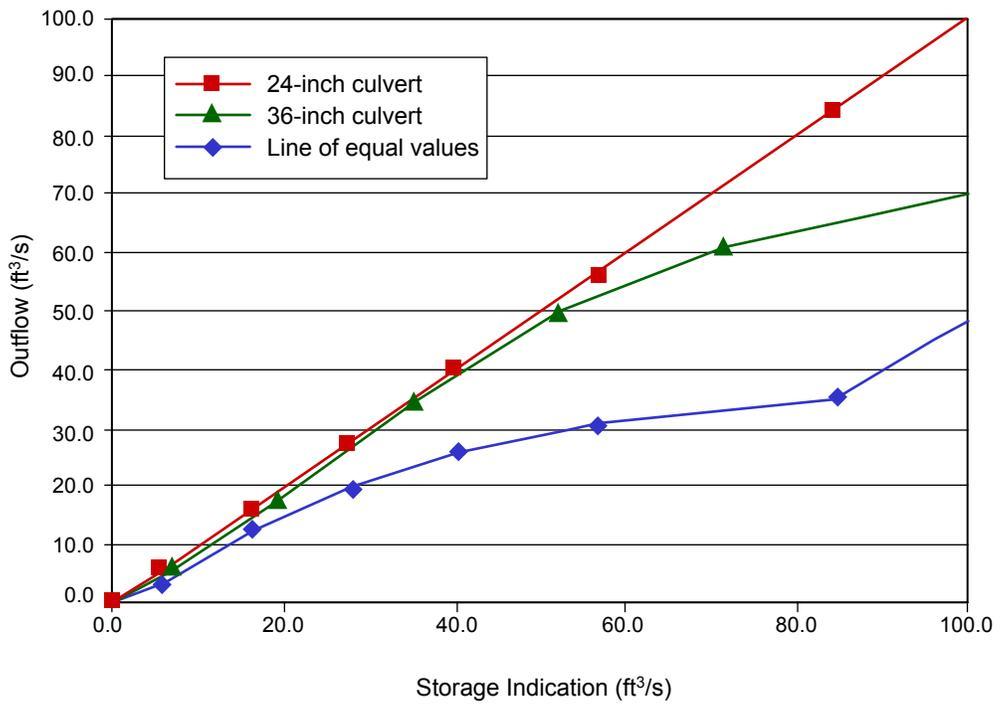
**Figure 7.3 (CU). Storage-indication curves for Example 7.2**
