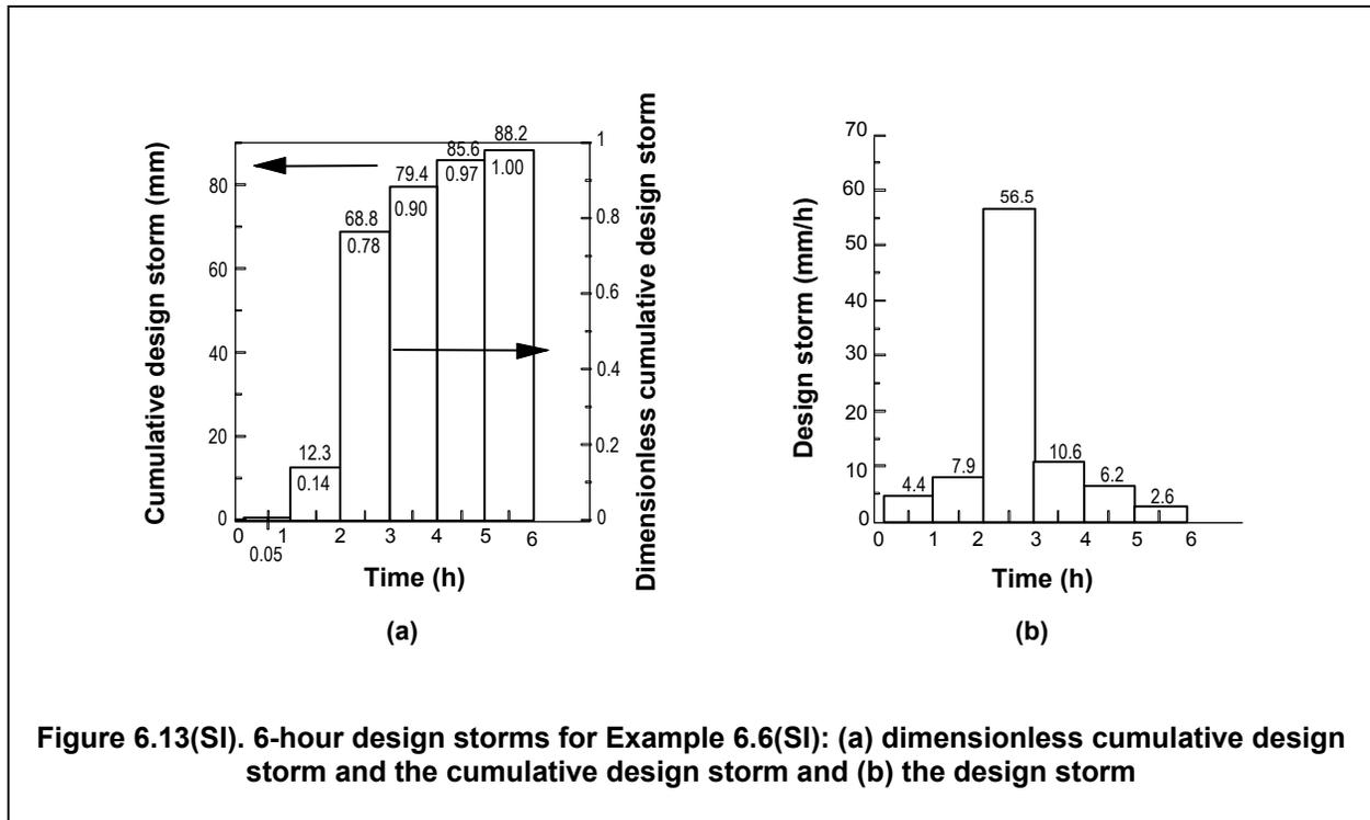
**Figure 6.13(SI). 6-hour design storms for Example 6.6(SI): (a) dimensionless cumulative design storm and the cumulative design storm and (b) the design storm**
