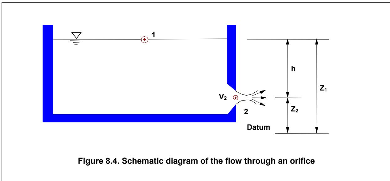
Figure 8.4. Schematic diagram of the flow through an orifice
