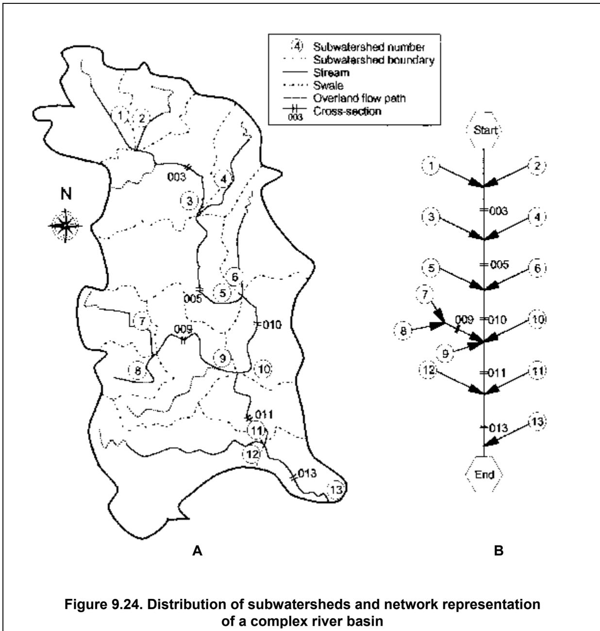
**Figure 9.24. Distribution of subwatersheds and network representation of a complex river basin**
