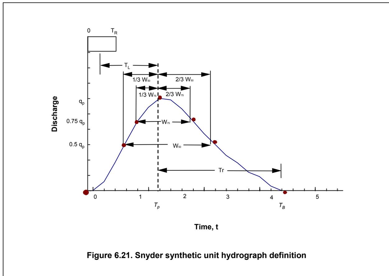
Figure 6.21. Snyder synthetic unit hydrograph definition
