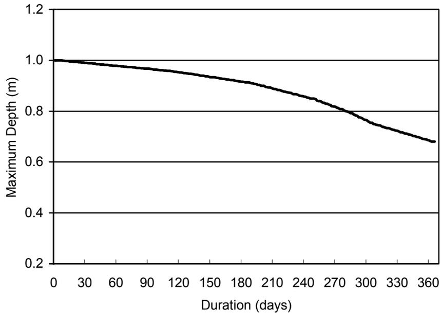
**Figure 9.12. Depth-duration curve for 1968 monthly water budget**
