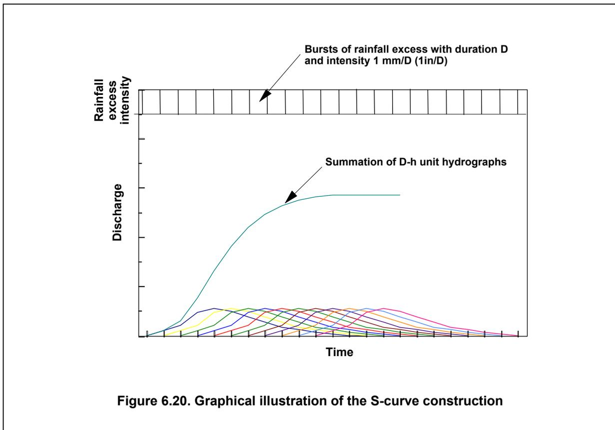
Figure 6.20. Graphical illustration of the S-curve construction
