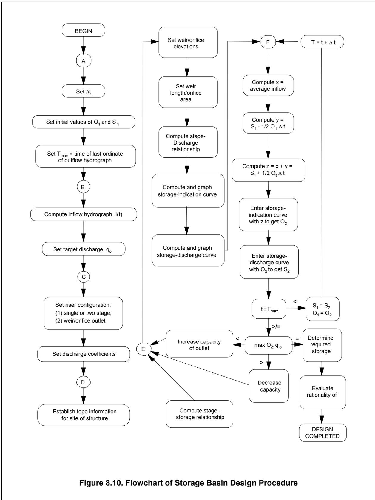
Figure 8.10. Flowchart of Storage Basin Design Procedure
