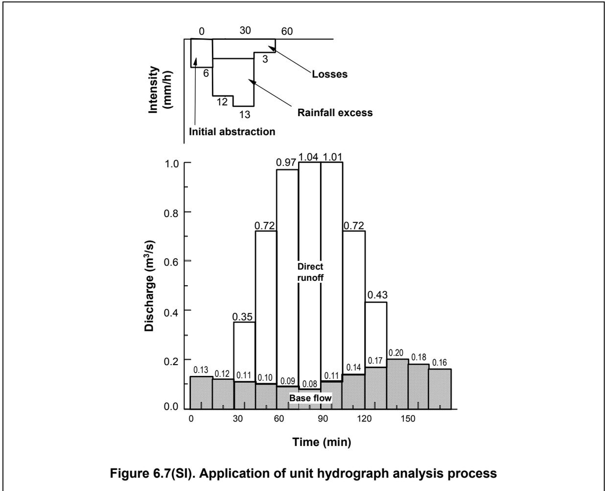
**Figure 6.7(SI). Application of unit hydrograph analysis process**
