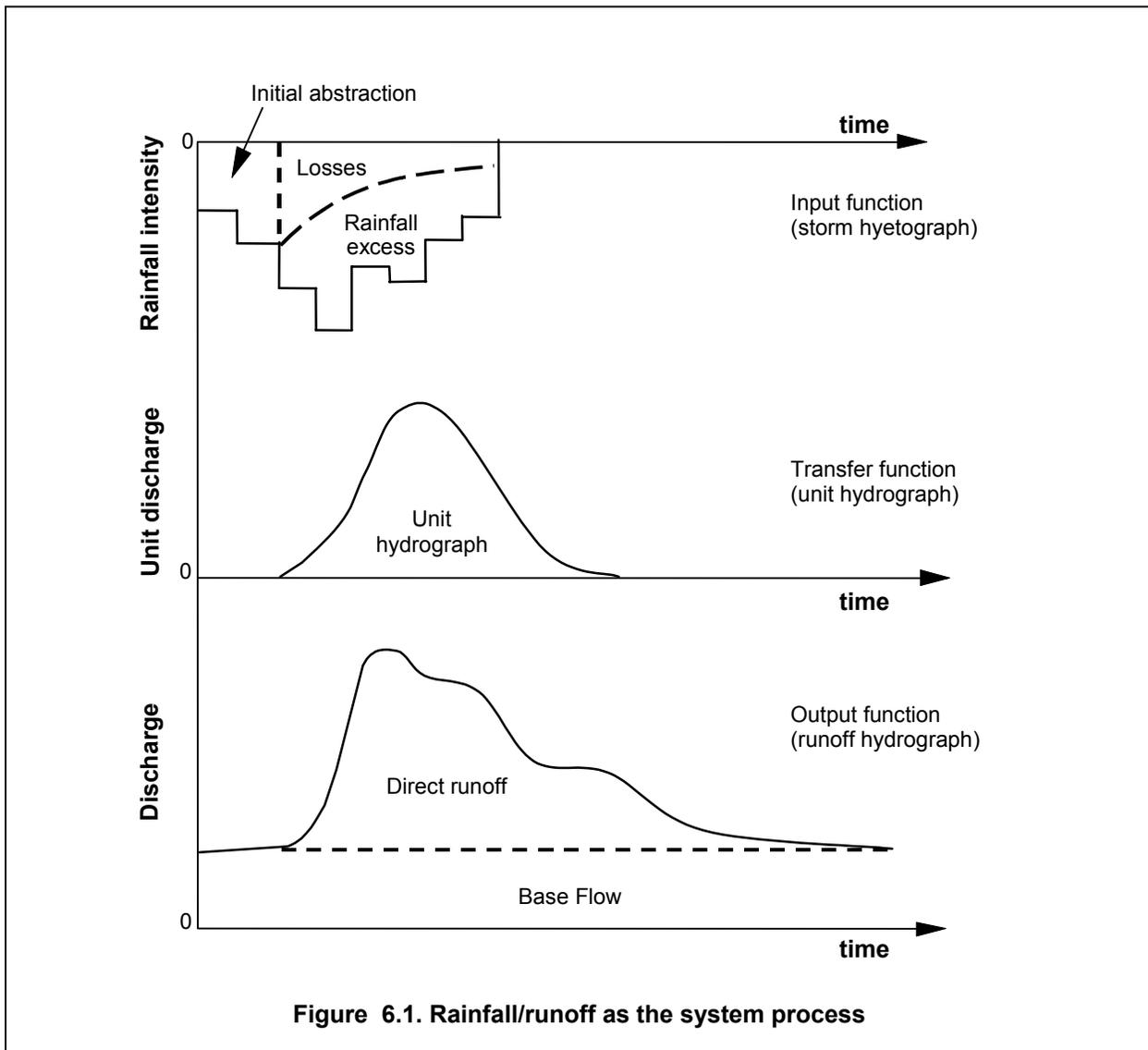
**Figure 6.1. Rainfall/runoff as the system process**
