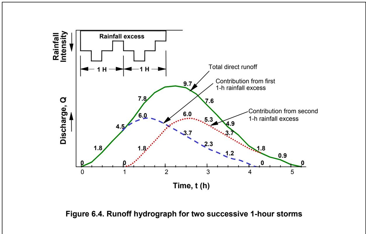
Figure 6.4. Runoff hydrograph for two successive 1-hour storms
