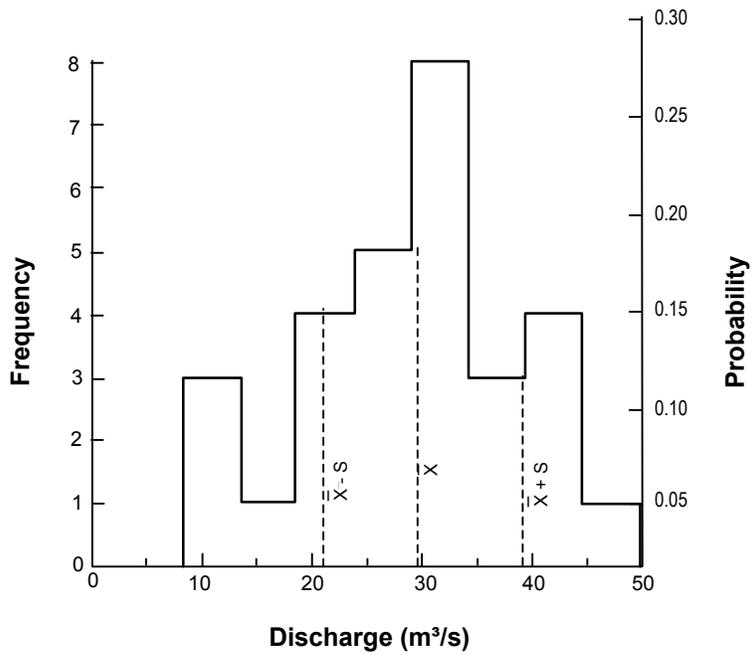
Figure 4.6a. Sample frequency histogram and probability, Mono Creek, CA
