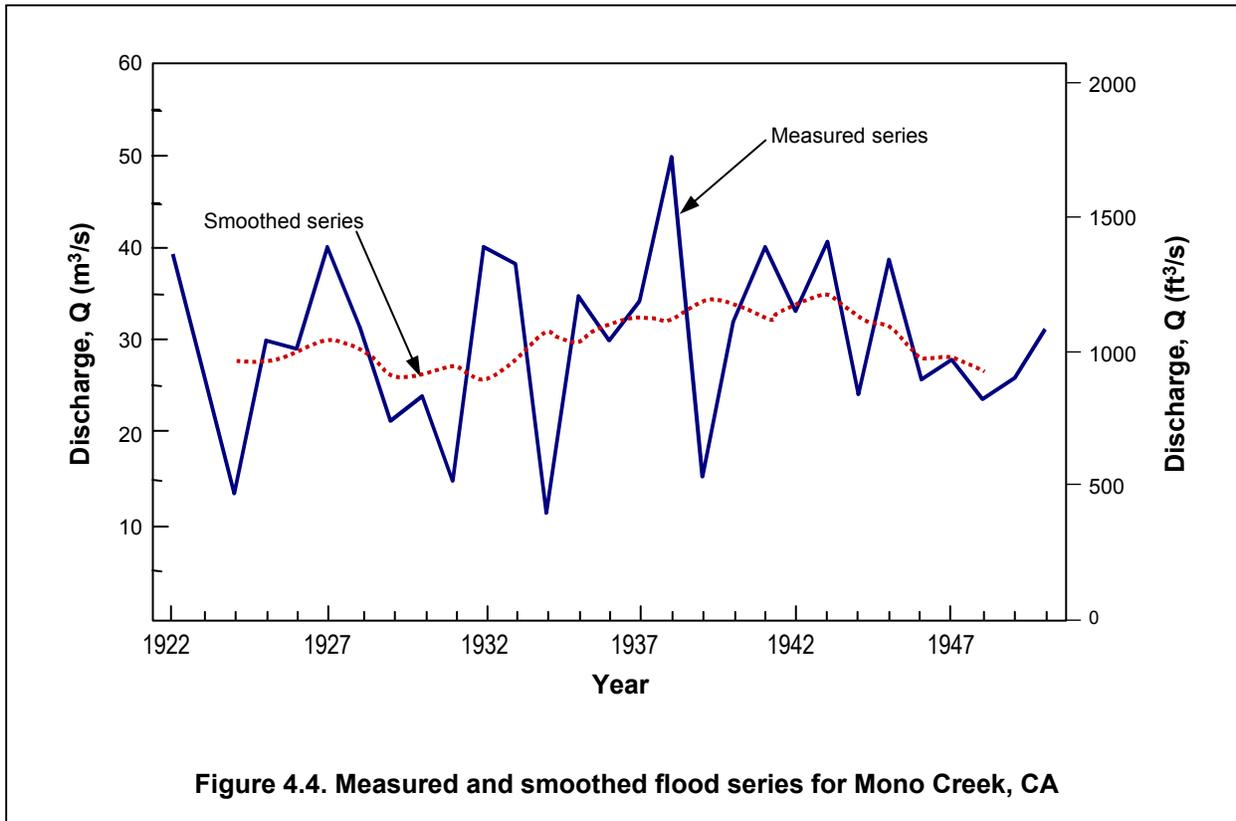
**Figure 4.4. Measured and smoothed flood series for Mono Creek, CA**
