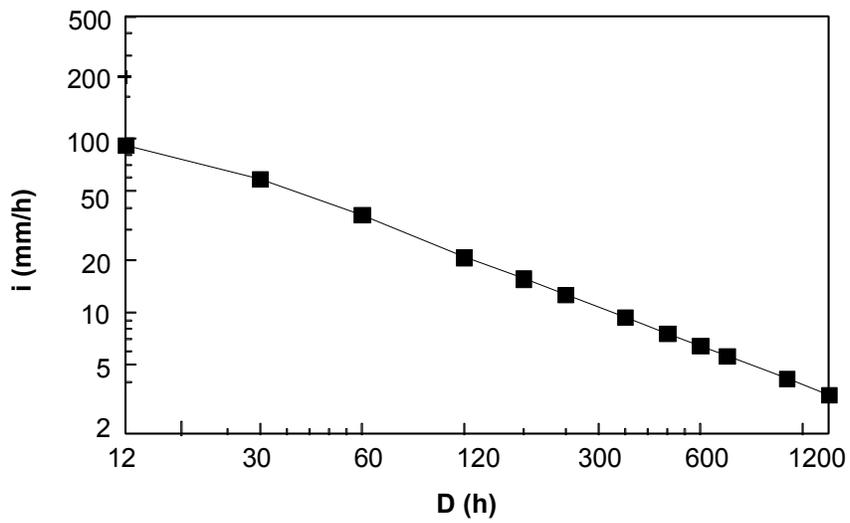
**Figure 2.15. Rainfall intensity-duration-frequency curves for selected return periods**
