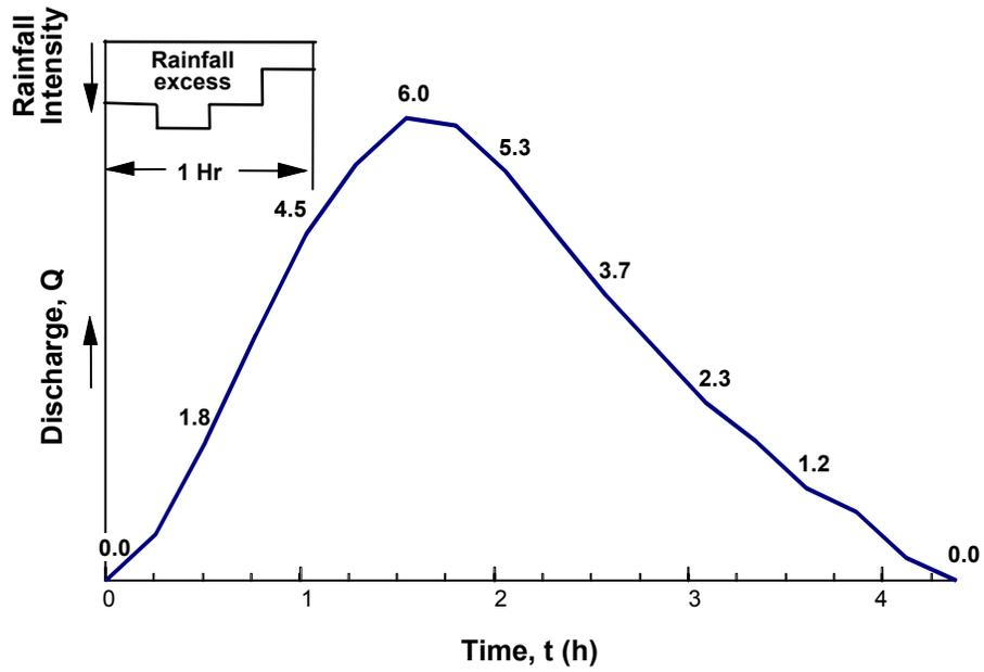
Figure 6.2. Runoff hydrograph for a 1-hour storm
