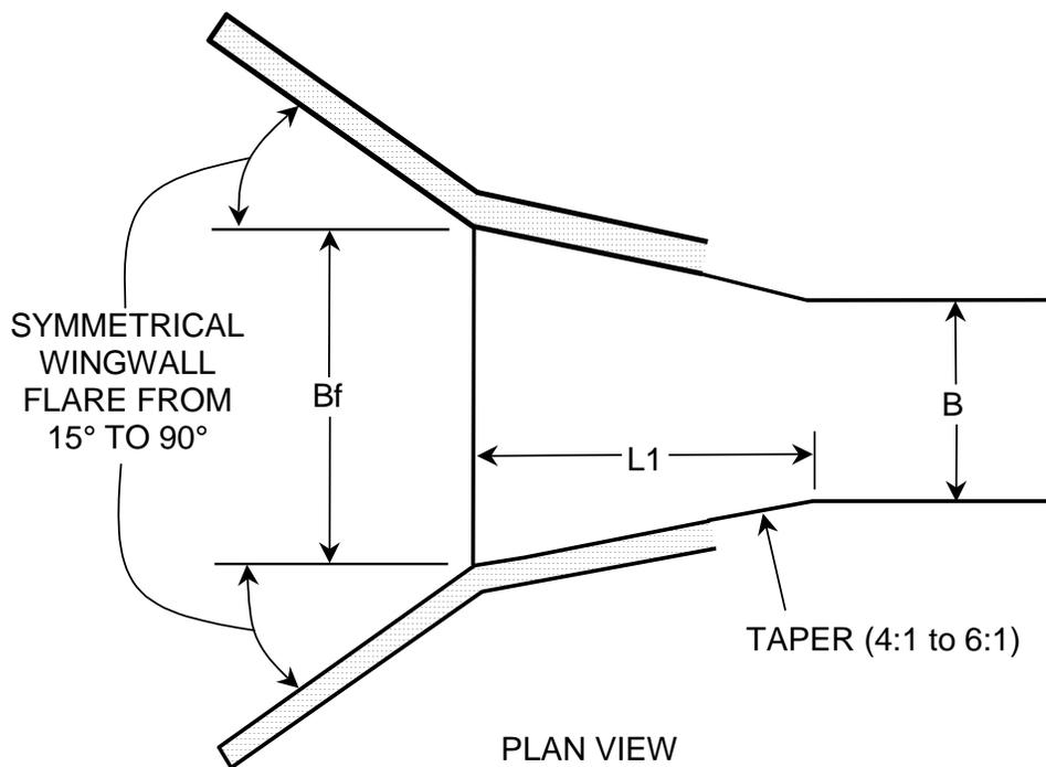
Figure 607-2 SLOPE - TAPERED INLET
