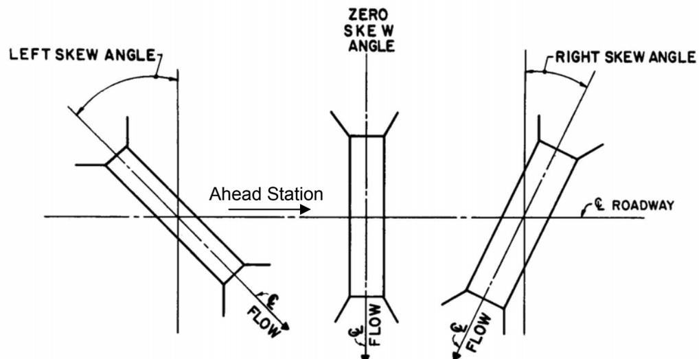
Figure 608-1 Culvert Skew
