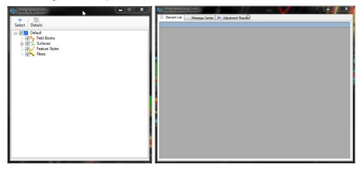
Right-click on "Surfaces" and select "Create Surface>Import External Surface>Import Lidar LAS". Now you can tell the program which LAS tiles to import.
