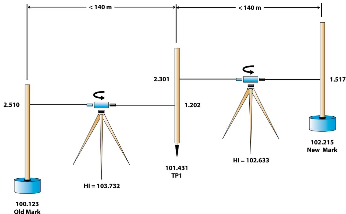
**8.** Compute the elevation of the new point, either the new bench mark or the turning point; this is the difference of the HI (computed in Step 5) minus the foresight.
