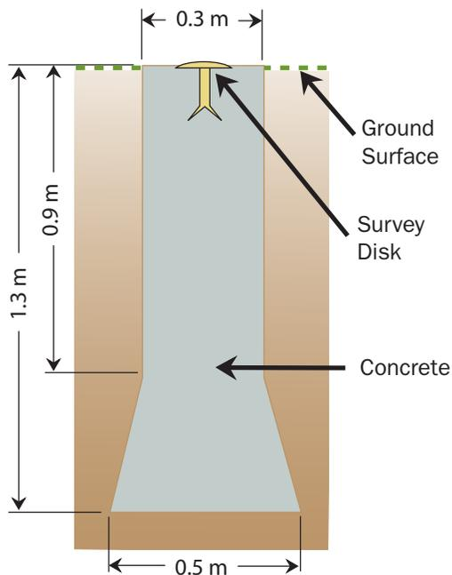
Figure B - 2. Schematic of concrete monument.
