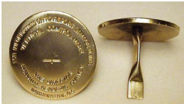
Figure B - 1. Brass disk, front and side view.
