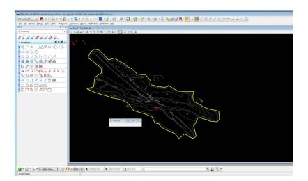
This has placed the offset feature, with elevations from the supplemental data, in our copy of the field survey data.
