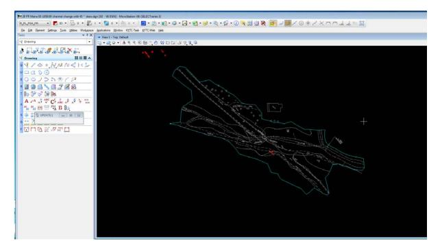
Next, select a value for the offset of the field survey boundary and perform the offset. For the example, 10' we will be used.
