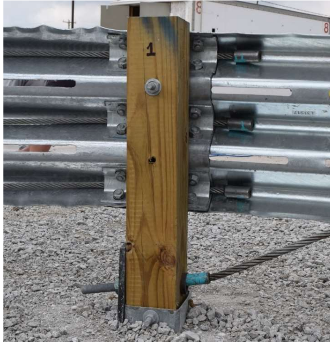
Figure 31 Nose Cable Attachment at Post 1
