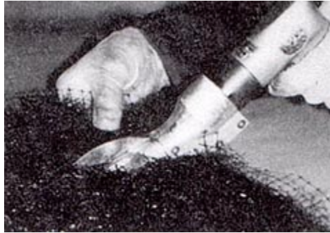
Hot Knife Specimen Preparation of non-degradable RECP.
