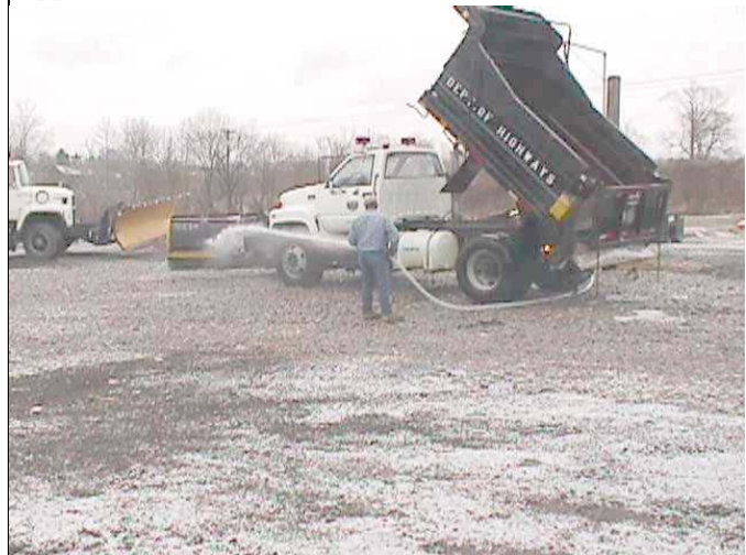
Clean trucks and equipment in location designated by the KPDES permit BMP Plan.
