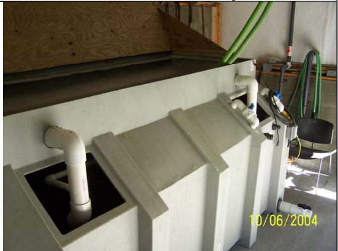
This new salt brine generator provides an environmentally sound method to generate brine.
