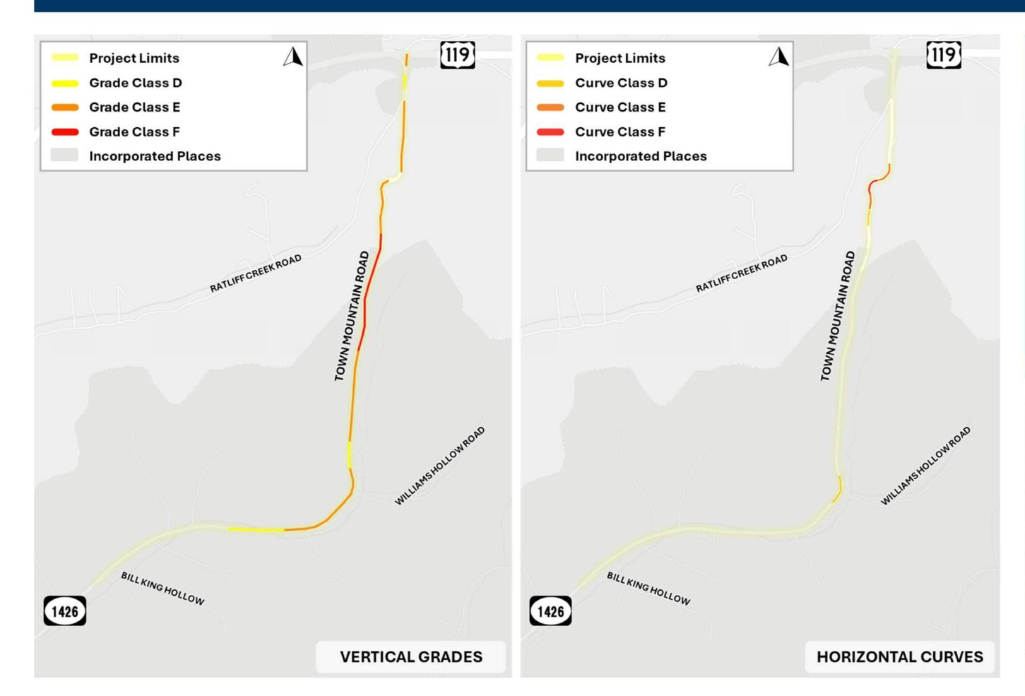
These conditions, coupled with narrow lanes (10-11feet-wide), minimal shoulders (less than 1-foot paved), and a short truck climbing lane (0.5-mile of the 2.5-mile corridor), contribute to reduced driving speeds and increased congestion, particularly when there are events at the Expo Center in Pikeville.
