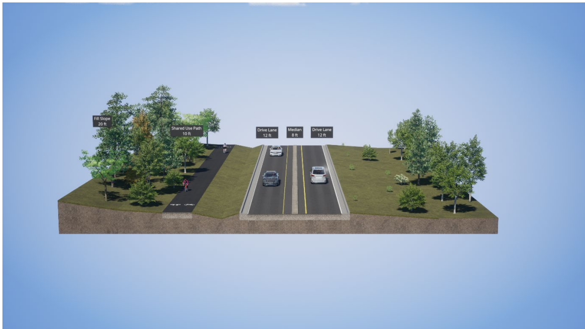
Proposed Roadway Typical Section
