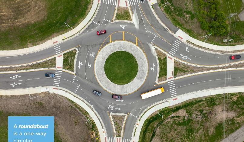
is a one-way circular intersection in which traffic moves counter-clockwise around a center island.
