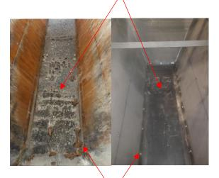
Skirting for aggregate conveyor on Micro Machine
