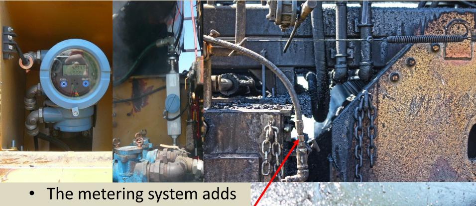
The metering system adds the emulsion based upon the mix design using a Mass Flow Meter.
