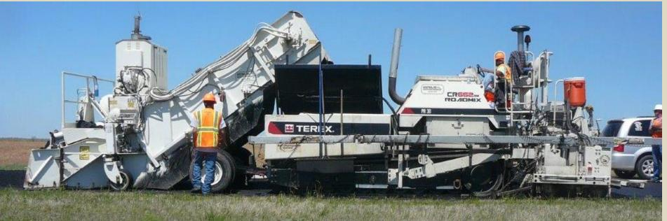
Dustrol uses a paver equipped with two counter-rotating augers that re-blend the material as it is delivered to the screed. This significantly helps reduce segregation of material.
