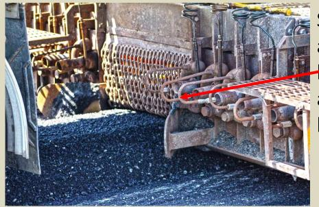
Special Tunnel heaters are used to allow the windrow to enter the heaters ovens. There the underlying asphalt is heated and the windrow is kept at temperature.
