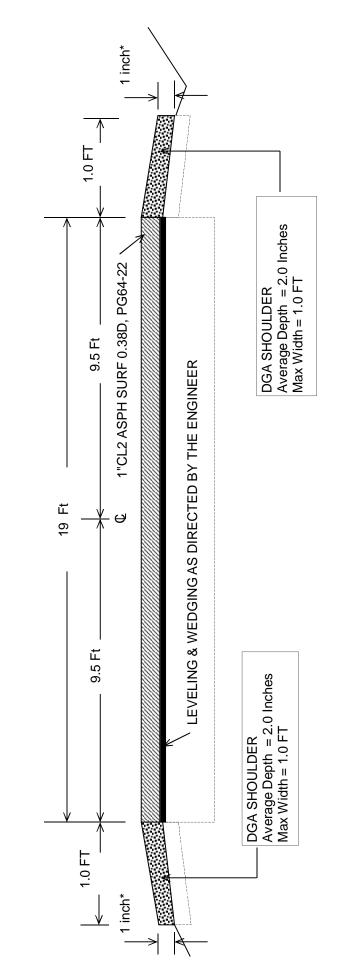
ASPHALT SEAL AGGREGATE AND EMULSIFIED ASPHALT RS-2 TO BE PLACED AT DIRECTION OF ENGINEER.
