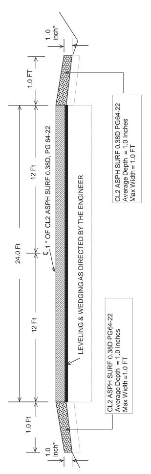
NOTE: STRIPING AS DIRECTED BY ENGINEER. DGA BASE USED ON OUTSIDE SHOULDERS AS DIRECTED BY ENGINEER; THIS IS TO REPAIR ANY DROP OFFS AT THE EDGE OF THE ASPHALT SHOULDER.
