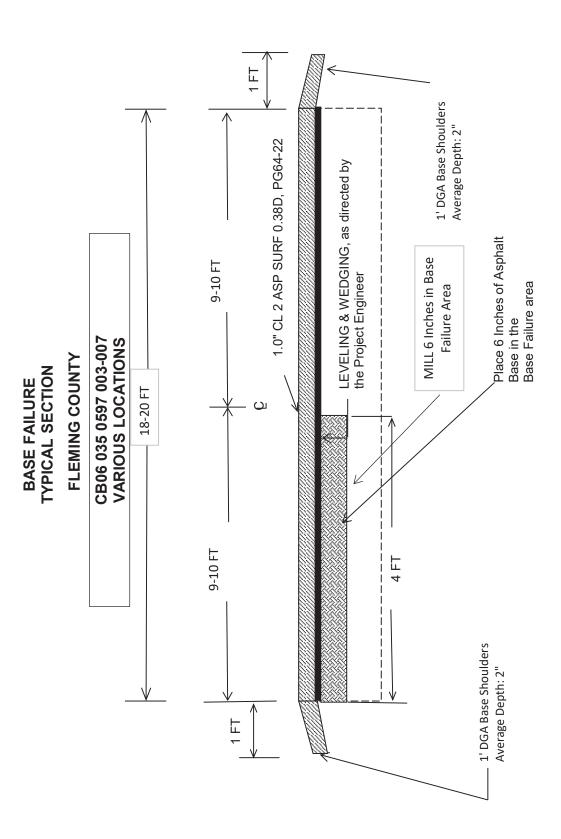
\*\* See Attached Sheet For Base Failure Repair Locations
