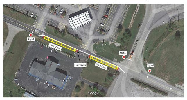
The remaining major base repairs can be constructed concurrently and should be constructed utilizing the following traffic control. Lanes shall be reduced to 10' widths and shifted to the opposite side of the roadway from the base repair. For all major repairs a quantity of temporary removable tape and barricades has been set up. All other necessary traffic control devices are to be incidental to maintain and control traffic.
