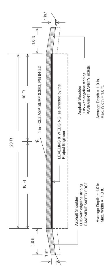
USE DGA AS NEEDED OR AS DIRECTED BY THE ENGINEER FOR SHOULDER DROPOFFS. \*Where Existing Site Conditions Permit
