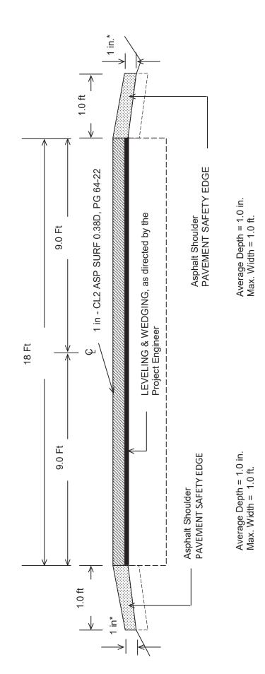
USE DGA AS NEEDED OR AS DIRECTED BY THE ENGINEER FOR SHOULDER DROPOFFS. \*Where Existing Site Conditions Permit
