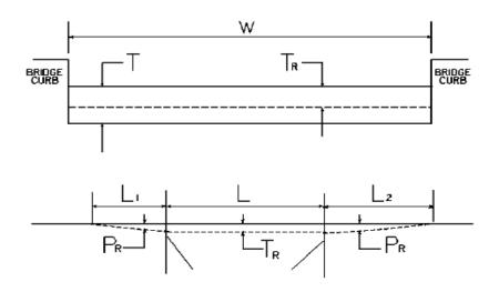
W = bridge width curb to curbT = thickness of existing bituminous overlayL = length of bridge $L_1 \& L_2$  = length of approach pavement to be removedP\_R = thickness to be removed and replaced on bridgeP\_R = thickness to be removed and replaced on pavementNote:  $L_1 \& L_2$  lengths shall be determined by using a transition rate of 100 ft / inch of thicknessFraction of thickness
