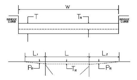
W = bridge width curb to curbT = thickness of existing bituminous overlayL = length of bridge $L_1 \& L_2$  = length of approach pavement to be removedTF $T_R$  = thickness to be removed and replaced on bridgePFNote:  $L_1 \& L_2$  lengths shall be determined by using a transition rate of 100 ft / inch of thicknessF
