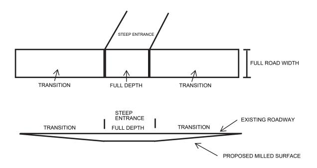
NOTE: THE TRANSITION LENGTH IS BASED ON 100 FT/INCH OF THICKNESS. NOTE: NO MILLING WILL BE REQUIRED IN THE ENTRANCES.
