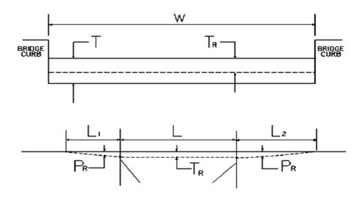
$L_1 \ \& \ L_2$  = length of approach pavement to be removed
