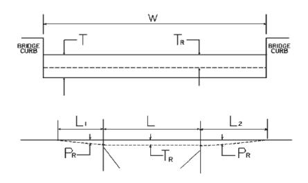
$\mathbf{W} =$  bridge width curb to curb T = thickness of existing bituminous overlay L = length of bridge $L_1 \& L_2 =$  length of approach pavement to be removed  $\mathbf{P}_{\mathbf{R}}$  = thickness to be removed and replaced on pavement  $T_R$  = thickness to be removed and replaced on bridge Note: L1 & L2 lengths shall be determined by using a transition rate of 100 ft / inch of thickness
