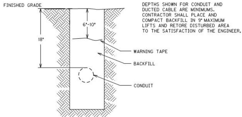
DEPTHS SHOWN FOR CONDUIT AND DUCTED CABLE ARE MINIMUMS. CONTRACTOR SHALL PLACE AND COMPACT BACKFILL IN 9" MAXIMUM LIFTS AND RETORE DISTURBED AREA TO THE SATISFACTION OF THE ENGINEER.
