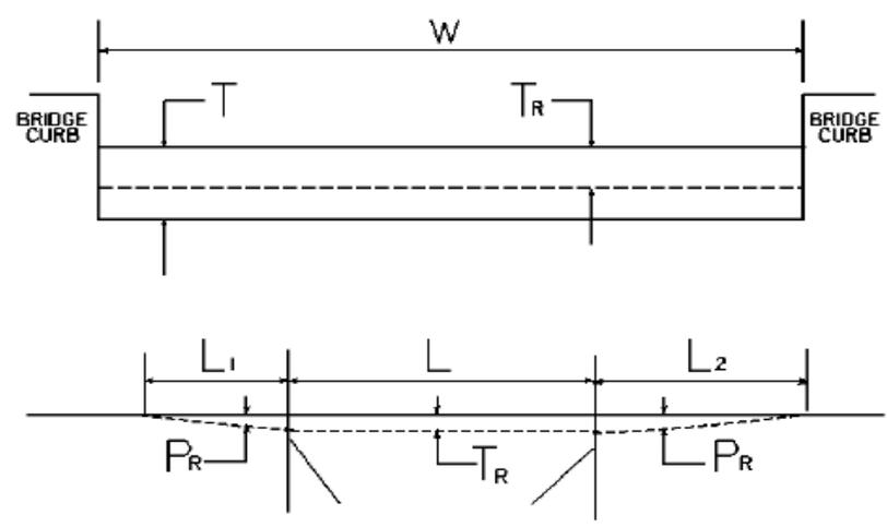
**W** = bridge width curb to curb                      **T** = thickness of existing bituminous overlay                      **L** = length of bridge
